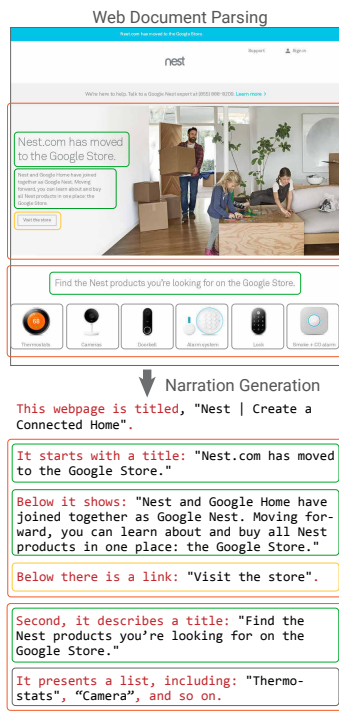
Figure 1: Designed for smart speaker users, our pipeline automatically creates narration for visually describing a web page based on the document structure. It connects key DOM elements in a narrative form that helps listeners better capture the content.
